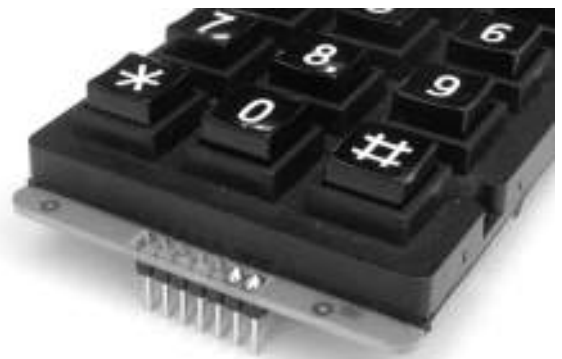
Figure 5-3 Soldering pins to the keypad.
