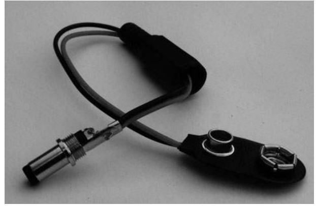
Figure 4-8 Creating a battery lead.
