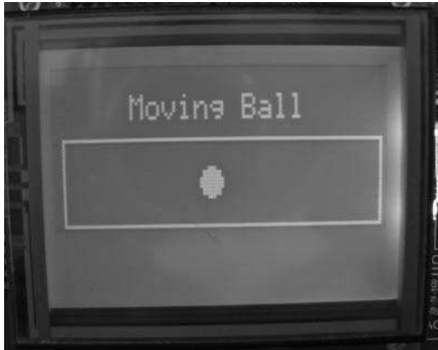
Figure 12.13 Created image displayed on the GLCD
