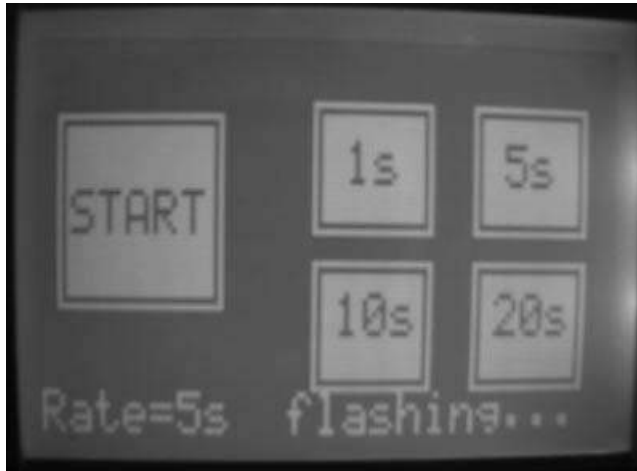
Figure 13.14 Display after starting the flashing action
