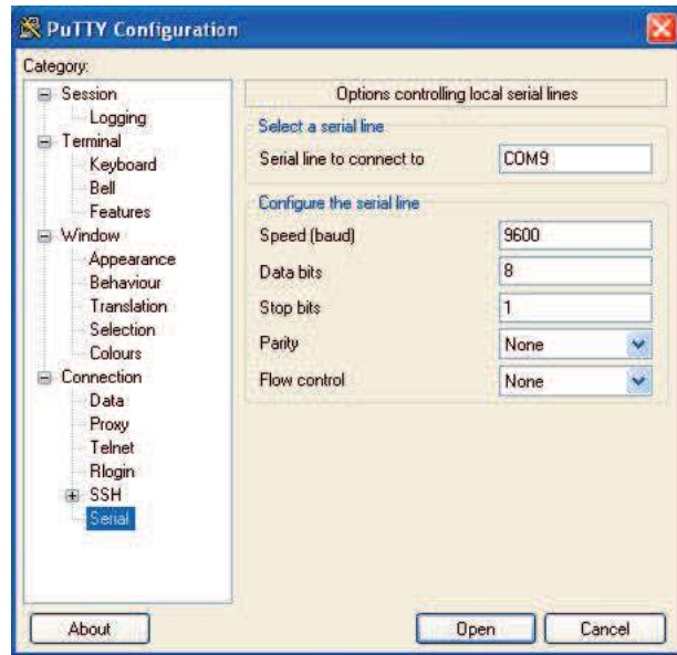
Figure 2.5: Configuring Putty to make it work with Arduino
