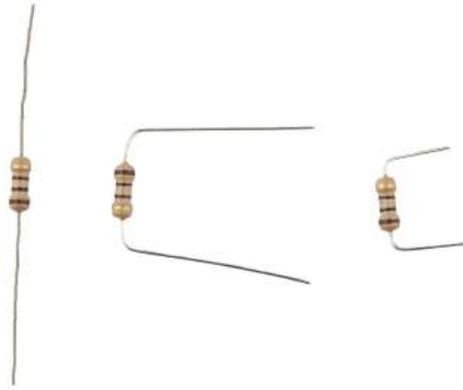
Figure 3.5: A resistor in various processing stages
