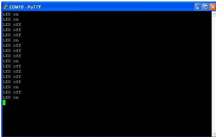
Figure 2.7: Putty communicates with Arduino.
