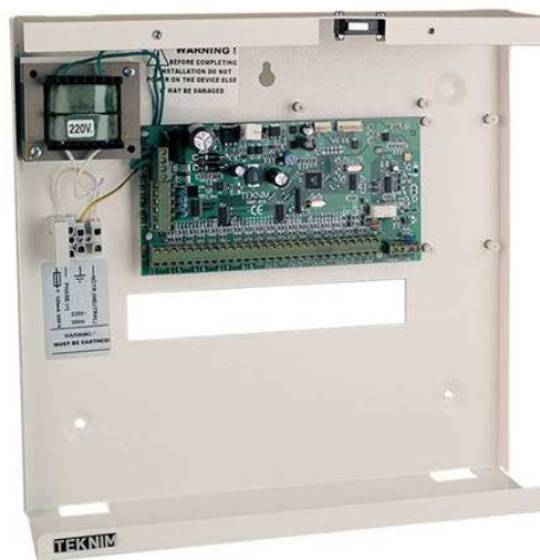
Figure 36: VAP-416 M ALARM PANEL
